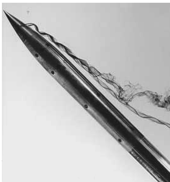
Fig. 5b Dye flow visualization of flow over an ogive cylinder at \alpha = 45 deg.
